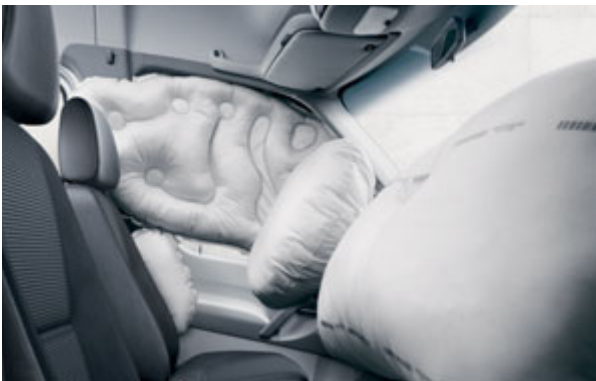
Window air bags and thorax air bags for the driver and front passenger are available as optional equipment. Various air bags shown at maximum deployment for illustrative purposes only.
