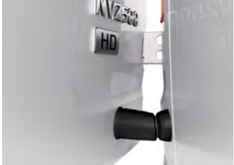
Powerful magnets hold the cargo doors securely in their fully open position.
