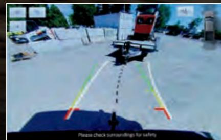
**REAR VIEW CAMERA WITH DYNAMIC HITCH ASSIST**
