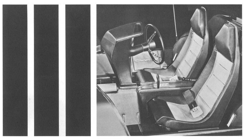
Pivoted, Contoured Bucket Seats. As the instrument cluster pod and steering wheel swing out of the way, the bucket seats automatically pivot forward and upward to add to the ease of getting in and out of Charger III. Looking much like acceleration couches from a space capsule, the contoured bucket seats with integral head restraints provide luxurious comfort and support.
