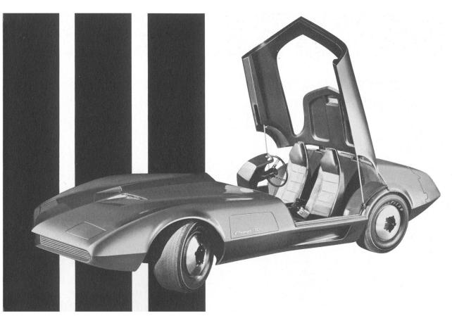
Raise-up Canopy. The entire superstructure of the passenger pod raises up smoothly and quietly with a concealed lift to make it simple and easy to get in and out of the extremely low Charger III.
