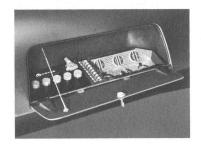
Engine Service Hatch. By opening the lockable engine service hatch located in the side of the fender on the driver's side, water level, oil level and battery fluid level can be checked without the need to raise the hood.
