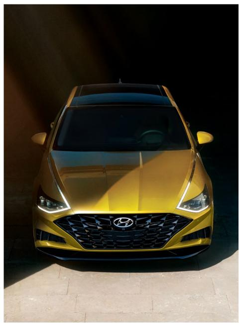
**Hidden innovation.** Our engineers created an unmistakable lighting signature unique to the Sonata that incorporates the very latest in lighting technology. Formed to the Sonata's body, the hidden LED daytime running lights appear chrome when turned off, and then dramatically brighten when turned on.
