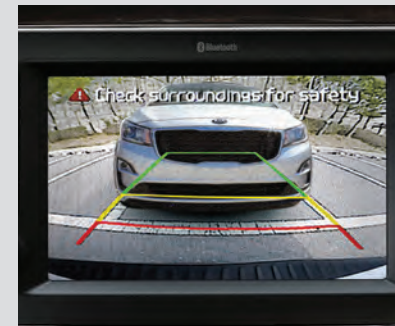
REARVIEW CAMERA 2 displays the rear view on your screen when you put your vehicle in reverse
