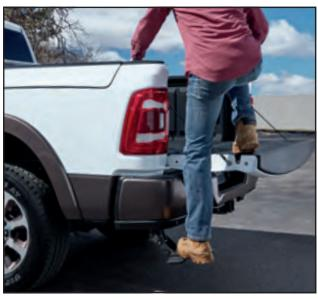
**BED STEP.** The available foot-actuated Mopar® Bed Step eases access to the bed and hides out of sight when not in use. Available as a factory-installed option or as a stand-alone Mopar Accessory.
