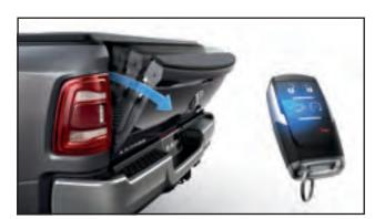
A BETTER TAILGATE. An available damped tailgate opens more slowly and closes with less effort. The tailgate also features an available power-release function; open it with the key fob button or via the in-cabin control.
