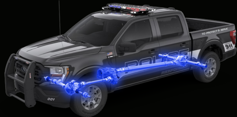
TORQUE-ON-DEMAND® 4x4 TRANSFER CASE
