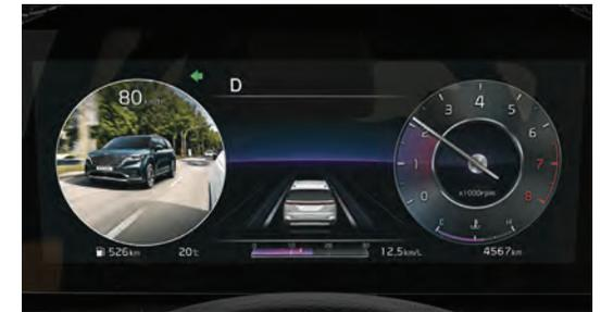
**Blind-spot monitor<sup>1</sup>** activates within the instrument panel when you turn on the blinker to change lanes, to display the blind spot in the direction of your turn signal.
