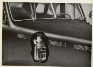
cowl, and operating the windshield wiper will clean the windshield without stopping the car.
