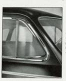
Roof mouldings and ventipane shields protect passengers from dripping
