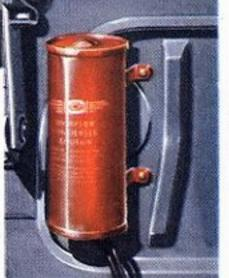
Reduces radiator coolant loss. Traps and liquefles steam, as well as trapping coolant overflow. Coolant thus saved is automatically siphoned back into radiator when cool.
