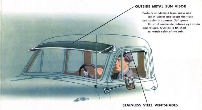
Ventshades that permit windows to be lowered in any weather for better ventilation and driving comfort. Reduce sun glare and window fogging.
