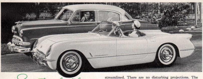
The low-set Corvette body expresses the swiftness that is so dramatically demonstrated by the car's performance. Taking full advantage of the new body material—glass-fiber reinforced plastic—Chevrolet engineers have created a sports car body in which all contours are smoothly
