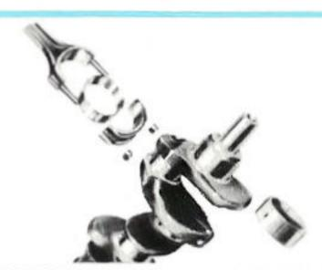
PRECISION INSERT BEARINGS are long-wearing, low-friction type, specially designed to withstand the stresses of heavy hauling. All Chevrolet Task-Force truck engines feature easily replaceable inserts on crankshaft main and connecting rod bearings.
