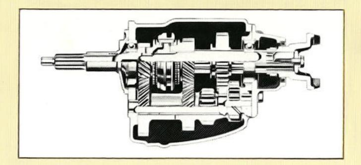
HEAVY-DUTY SYNCHRO-MESH 4-SPEED is the trucker's favorite for heavy service. Simple, rugged, and dependable with powerful 7.06:1 low gear ratio. Synchro-Mesh design eliminates double clutching. Standard on 1-ton, optional on 1½- and ¾-ton pick-up models.
