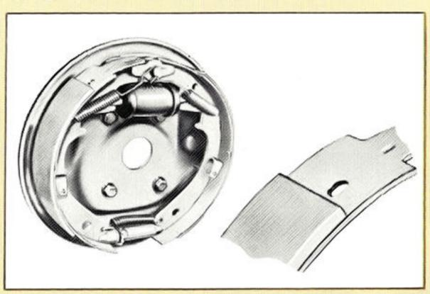
TORQUE-ACTION BRAKES produce safe, positive stopping power with light pedal action. Brake shoes are energized by wheel rotation. Bonded linings on pick-up models nearly double brake-lining life.
