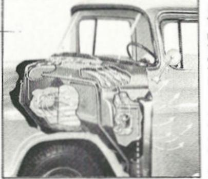
TILATION—another mark of a truly modern truck—supplies fresh outside air, offers efficient air circulation in all kinds of weather. Intake is located beneath the windshield to minimize road heat, fumes, and dust. Individual controls for driver and passenger permit separate control of fresh air supply.
