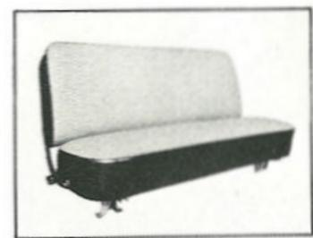
NU-FLEX SEAT is designed for relaxed riding on roughest roads. Seat is covered with durable, easy-breathing fabric. Foam rubber cushion is optional in De Luxe cab, standard on Custom cab.
