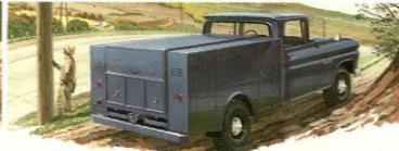
\* CHEVROLET CHASSIS-CABS readily adapt to a wide range of special bodies like this service-utility body. New four-wheel-drive equipped models K1403 and K2503 have the hauling capacities, the pulling power, and ground clearance to get over rugged terrain with heavy loads.
