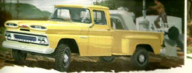
CHEVROLET STEPSIDE PICKUPS for 1960 are available in two 4-wheel-drive models—K1404 and K2504—with box lengths of 78" and 98". They feature graintight tailgates, select wood floors with recessed steel skid strips, convenient running boards, and stake pockets for racks or sideboards.
