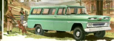
CHEVROLET SUBURBAN CARRYALLS in the 1960 4-wheel-drive lineup are ideal for many jobs that combine passenger transportation with cargo hauling. Seating accommodates eight. Seats can be quickly removed. Model K1406 has panel rear doors. Model K1416 has tailgate and liftgate.
