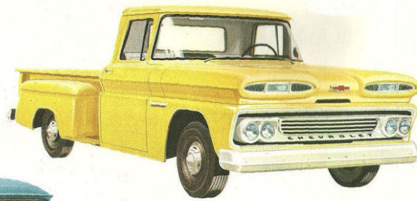
STEPSIDE C1404 —Here's one of Chevrolet's 1960 Stepsides with select wood floor and grainless tailgate. Convenient running boards make side loading a cinch. It's designed for a maximum G.V.W. of 5,200 lbs. Floor area is 78" long, 50" wide.
