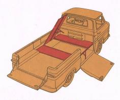
Optional\* level load floor is also available for Rampside models, with ramp door offering convenient access to protected sub-floor stowage space.
