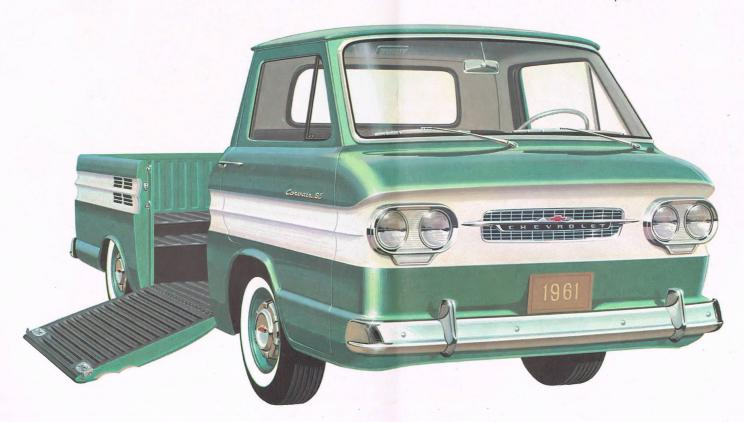
Here's something new and exclusive in pickups—cargo-handling ease without precedent in the field! A rugged-built cargo ramp swings down flush with the floor of the deep-well load compartment, leaving a gateway nearly four feet wide to get big loads in and out without lifting. With the floor less than 14 inches
