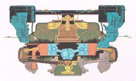
FORCED-AIR COOLING controls engine temperature efficiently and directly, without the intermediate stage of a liquid coolant which must be air-cooled in a radiator. A high-capacity blower blasts cooling air between cylinder barrels and through passages in the heads, where it picks up heat directly from deep, efficient cooling fins. A thermostatically controlled ring damper governs the air supply to the blower, speeding engine warmup and stabilizing operating temperature automatically.
