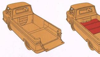
Nearly 28 inches deep, the Loadside's deep-well cargo area accommodates tall, bulky loads with ease. Weight is carried low and amidships for superior handling over the road.
