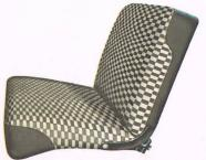
Corvair 95 seats are built on Chevrolet's steady-riding combination spring frame design, with S-wire, coil and flat spring elements combined to bring out the best features of each type. Thick foam cushions top the springs in the De Luxe seat (illustrated) and an extra-thick foam seat cushion plus a foam backrest cushion are included with the Custom option.\* Standard seat in the Corvan is single-width, for driver only, with a full-width seat optional at extra cost.
