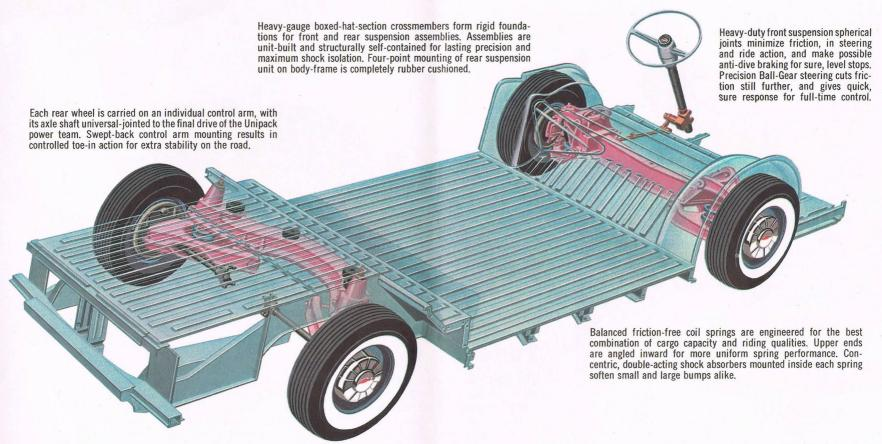
The Corvair 95 fully independent suspension system brings matchless ride and handling to light-duty truck design, coupled with truck-engineered load capacity and durability. Precise control of each wheel's action results in exceptional engineered-in roadability, for sure-footed performance on any road. Front and rear suspension assemblies are built up on rugged boxed-hat-section beams, which give broad-based support to the body frame-floor assembly. Friction-free coil springs at all four
