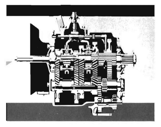
In addition, the Spicer five-speed, close-ratio 5756B transmission, formerly offered only with Series 80 Diesels, is now available on conventional, LCF and Tilt Cab Series 80's, when used with the 409-V8 gasoline engine or 6V-53 Diesel.
