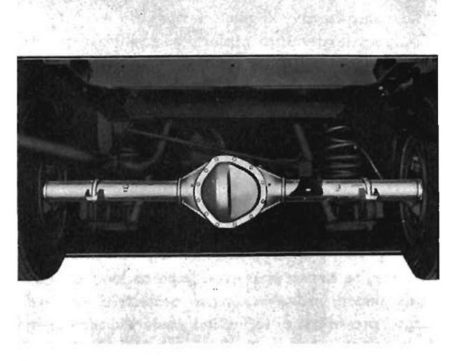
Stronger, quieter Salisbury-type rear axles for Two-Wheel-Drive Series 10 models also are new this year. Built-in ribs on the cast differential carriers, combined with steel tube axle shaft housings, provide new rear-end strength and durability.
