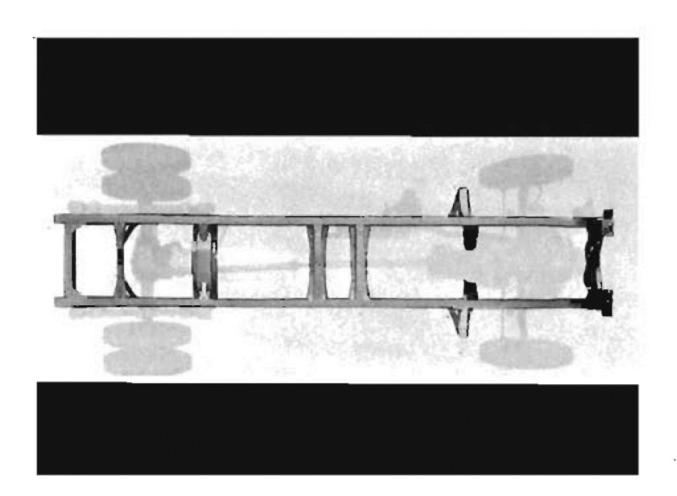
Medium- and heavy-duty models feature new, full, ladder-type, channel-section frames. Heavier-gauge siderails and improved cross member design make these new frames stronger than ever. On most models, siderail metal is substantially thicker—.093 of an inch thicker. This new frame strength provides increased load support and greater durability.
