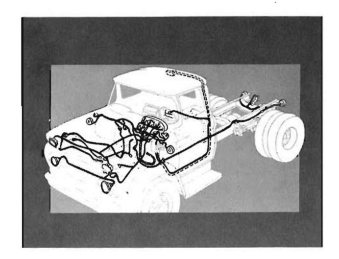
Engine wiring subject to overloading or abuse is protected by a special nonmelting synthetic rubber insulation. It is used on chassis and engine wiring harnesses on D60, 60-H and 80 Series models. Wiring failure is a frequent cause of truck down time.
