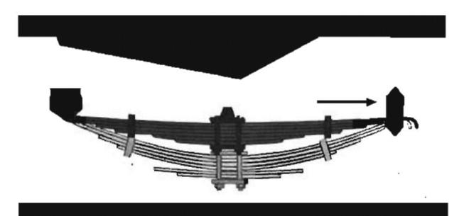
With heavier loads, the top leaf shortens, providing increased load support plus comfort. Engineering and on-the-road tests prove this to be the most ideal suspension ever offered on heavier-duty trucks.
