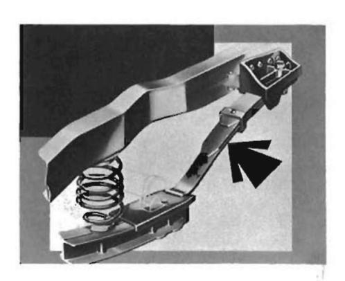
New three-leaf auxiliary springs are available optionally on Series 10 and 20 models. These auxiliary springs do not affect ride and handling characteristics under light loads. Under heavy loads each spring adds 500 lbs. carrying capacity and rear-end stability is improved.
