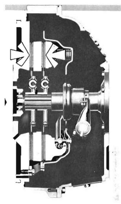
A new, two-plate, 12-inch clutch provides a perfect match for the 409-V8's High Torque power output.
