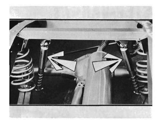
On light-duty models, rear shocks have been repositioned for more positive ride control. Rear shock absorbers are now attached to the frame ahead of the rear axle. At this location, body motion transmitted to the shocks is more easily absorbed.
