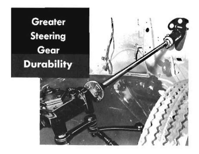
STEERING—A new single-piece steering gear shaft replaces the multiple-piece type formerly used. Steering gear linkage has also been simplified for maximum durability and optimum steering characteristics.
