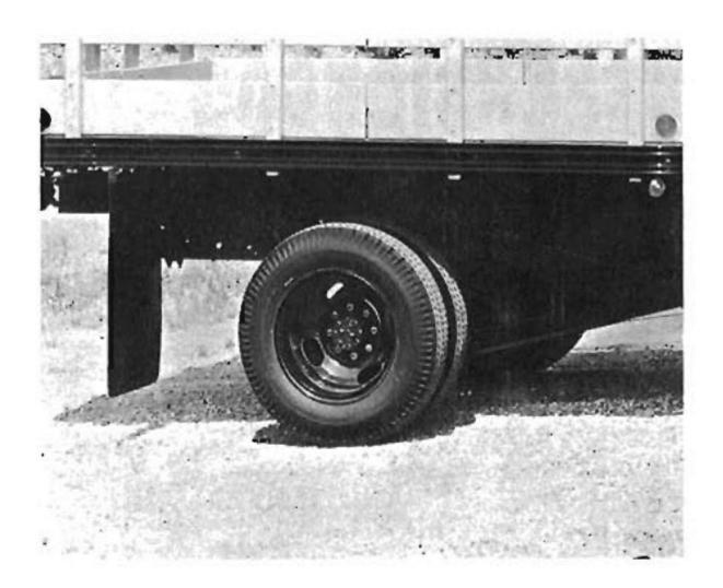
For the first time, 16-inch dual wheels are available on Series 20 models for extra load-carrying capacity, traction, flotation and lower loading height.
