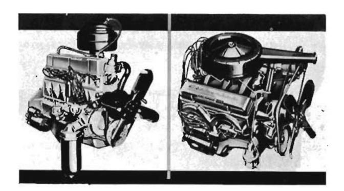
Two optional engines are available on regular light-duty trucks. They are the new 292-cubic inch Six, standard on Series 60 and 60-H, and the improved 283-cubic inch V8 which, with redesigned cylinder heads and increased compression ratio, delivers more horsepower on regular gas.
