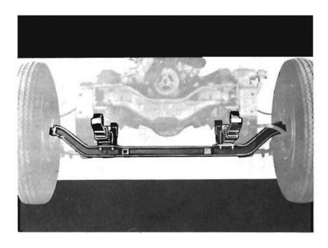
The new frames are supported by the newest and best suspensions in the business. I-beam axles with variable-rate front springs are standard equipment. Variable-rate springs have been proved over millions of miles on rear suspensions. Now, for the first time, they are available on front suspensions. They provide reduced maintenance, better tracking and superlative ride and handling qualities.
