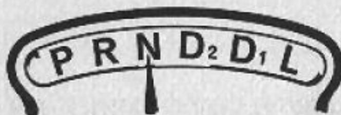
P — Park. Locks the rear wheels safely and positively. Convenient for starting the car on a grade.
