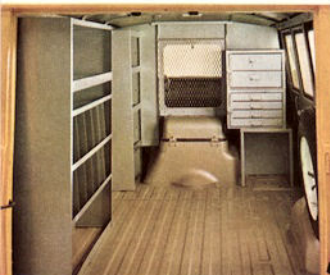
Cabinets and bins for general delivery and repair service
