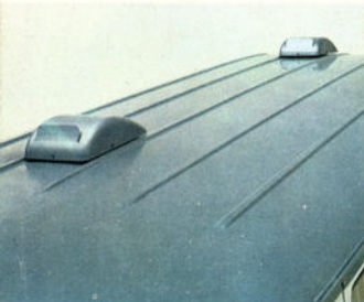
Twin air vents
