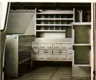
Cabinet and bins for plumbing, heating and air conditioning service
