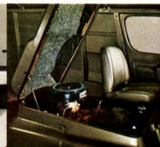
Heavily insulated engine compartment
