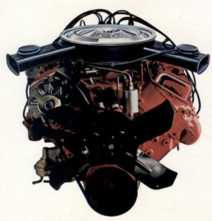
270-horse 350-cubic-inch V8 that inhales through a 4-barrel carb and exhales through dual exhausts. If you
