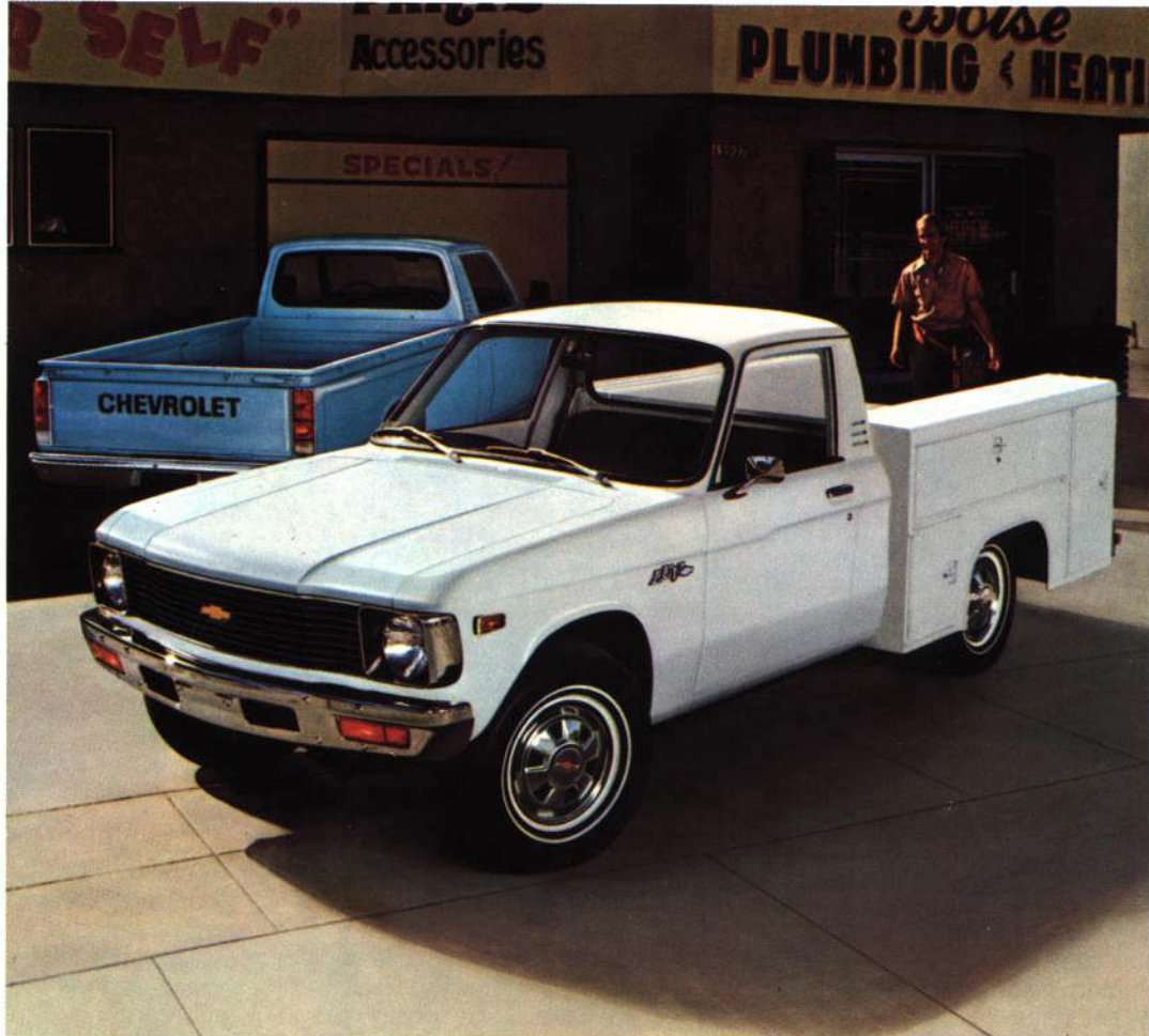
Chevy LUV chassis cab model is available in the 102.4-in. wheelbase to allow installation of special equipment including utility bodies as shown above.
