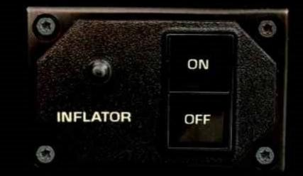
A unique feature of the STE is the Inflator mounted in the trunk. Working off the air-pressure system for the Electronic Ride Control, this unit can be used for checking tire pressures, or inflating recreational equipment.
