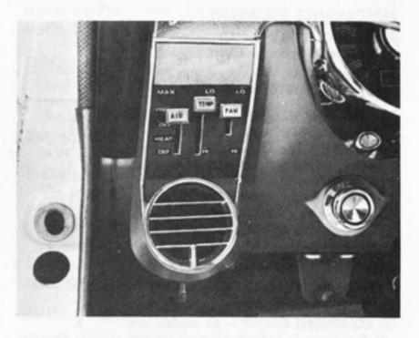
SELECTAIRE AIR CONDITIONER — The Select-Aire air conditioner is a deluxe unit fully integrated into the instrument panel and heating system. It is designed to provide year-round passenger comfort, obtained from one set of controls.
