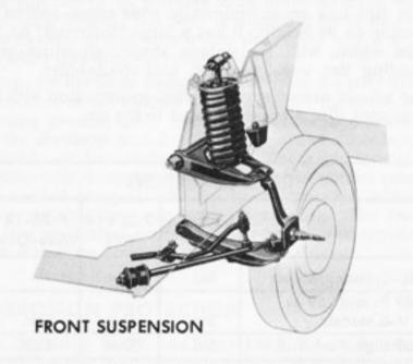
A unique option available on the Mustang is the heavy-duty suspension which includes increased rate springs, larger and recalibrated shock absorbers, and increased diameter stabilizer bar. This option provides increased roadability and handling.
