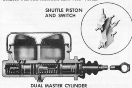
As an added safety feature, an instrument panel warning light will go on if a pressure loss occurs in either half of the system. The light is connected to a shuttle piston between the front and rear brake lines. Normally, the shuttle piston does not move. But, should a pressure loss occur in either brake system, a significant differențial in pressure results and the shuttle piston activates a switch that turns on the warning light when brakes are applied.
