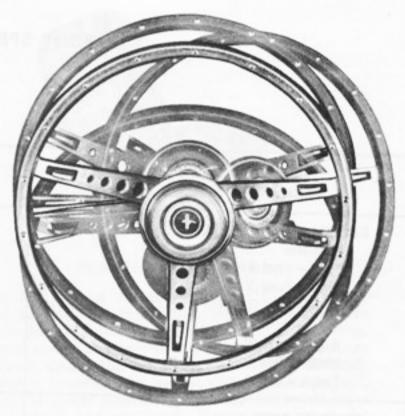
shift lever in "Park," opening the driver's door swings the column up and to the right at a 45-degree angle, providing maximum entry/exit room. After re-entering, and with the door closed, the driver pulls the column back and it locks in position. A built - in "memory" always returns the wheel to the previously adjusted tilt position.
