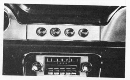
CONVENIENCE PANEL — Available for the first time on the '67 Mustang is the convenience panel that includes warning or reminder lights for door ajar, parking brake, low fuel and seat belts. The panel is installed on the instrument panel above the radio or on the optional console.
