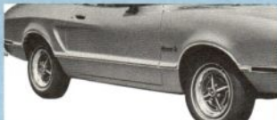
Vinyl-Insert Bodyside Molding —Color-keyed and integrated with side marker lights
