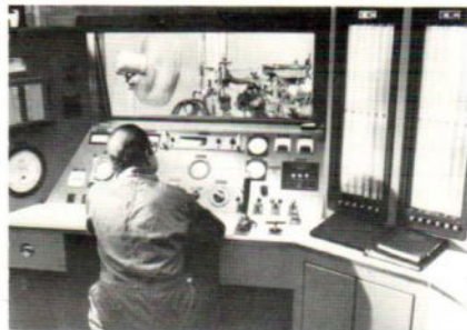
Selected Engines Test Run up to 150 Hours
