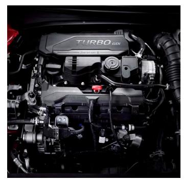
**Standard Smartstream 1.6L Turbocharged GDI engine**The ELANTRA N Line's Smartstream 1.6T GDI engine delivers
