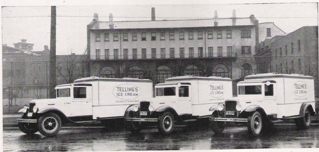
Three of a fleet of 34 new Internationals recently delivered to the Telling-Belle-Vernon Co., of Cleveland. These special-built ice cream bodies are of 400-gallon capacity.
