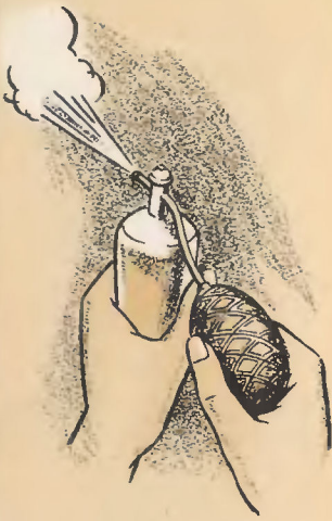
The action of a carburetor is much like that of sister's or mother's perfume atomizer.
