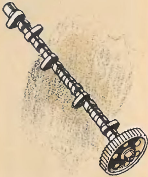
Knob-like projections on the camshaft make the valves work.
