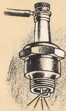
The spark plug causes electric sparks to set off the explosions.
