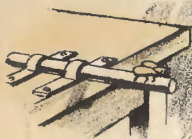
A fly's weight bends a steel bar one-millionth of an inch.
