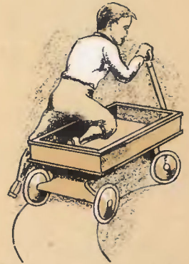
When turning a corner the outside wheel must go farther, therefore faster.
