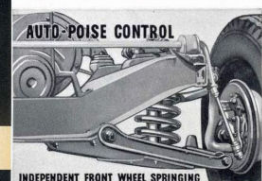
INDEPENDENT FRONT WHEEL SPRINGING
