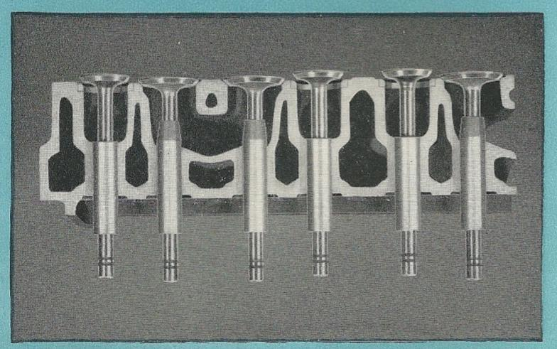
This cross section through part of the **Green Diamond** engine block shows the large water passages which completely surround intake and exhaust-valve ports; the large exhaust-valve ports which facilitate the escape of hot exhaust gases; the heavy-duty, truck-type intake and exhaust valves; and the hardened exhaust-valve seat inserts.
