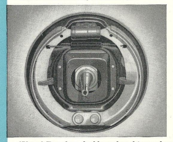
(Above) Two-shoe, double-anchored internal-expanding hydraulic brakes provide smooth, straight-line stops and braking effectiveness on all wheels with light pedal pressure. The two braking shoes are supported on the backing plate by two fixed anchor pins at the bottom of the brake.
