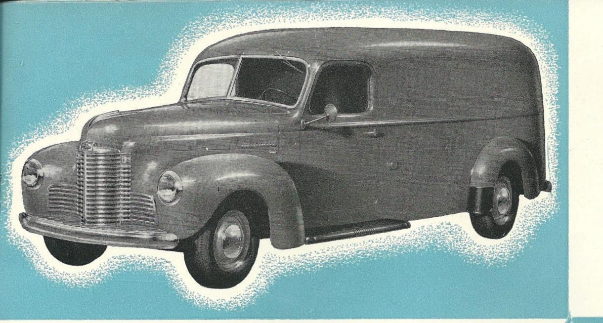
Handsome, large - capacity International streamlined de luxe panel bodies are rigidly constructed for safety and long life. The trim, symmetrical lines are further enhanced by the pressed-in belt and panel moldings. The panel body has a capacity of 171 cubic feet and measures 109 \(^3\)\% inches long at the floor, 46 \(^3\)\% inches between wheel housings and 56 inches high.
