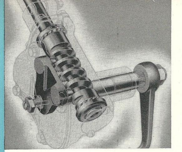
Safety at all speeds and easy steering under all road and load conditions are assured by the use of the cam-and-twin lever steering gear. The entire steering mechanism is fully enclosed in oil and dustproof housing.
