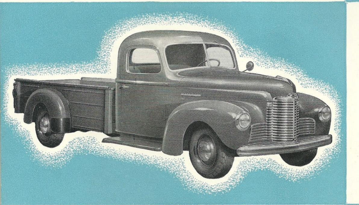
Pickup bodies have exceptionally large load capacities. The lines of the long all-steel dropskirt bodies blend with the graceful contours of the grille head, cowl and cab, forming a light-duty transportation unit of distinctive appearance and maximum utility. Loading space is 102 inches long,  $48\frac{1}{2}$  inches wide and 17 inches high at the top of the 4-inchwide flareboards.
