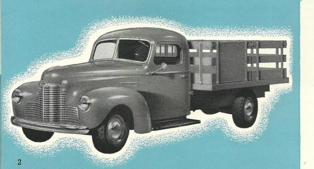
An 8-foot, light-duty, panelstake body with 14-gauge welded steel understructure and thoroughly seasoned oak floor is available for the 130inch wheelbase Model KB-3 chassis. The one-piece front section and the two-piece side sections are removable and are fitted to the top with interlocking connections. Inside measurements are 96 inches long, 78 inches wide and 30 inches high.
