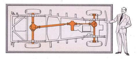
On smooth roads or level ground, you operate a 4-wheel-drive vehicle just like any other car with a standard shift. When necessary, just flick a lever and change over to 4-wheel drive. A special low gear-range gives extra pulling power for emergencies, assures you
