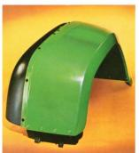
Cab fenders attach with eight bolts and lift away quickly for walk-up accessibility to the engine. Handy for routine maintenance. Relatively inexpensive to replace in case of accidental damage.
