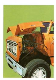
Butterfly type side opening hood swings up and out of the way for easy access to engine, oil filter, dip stick and radiator cap conveniently located for fast checking. Front fenders and entire hood assembly remove in a matter of minutes. Standard on all 7500 models.
