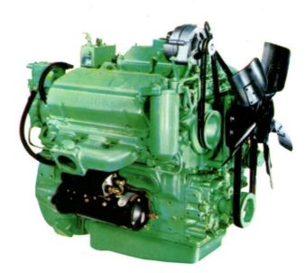
Detroit Diesel power can make the difference you want. 6V-53N and H engines offer design features that include precision needle valve injectors; low pressure fuel transfer pump that eliminates high pressure fuel lines; Posi-Temp cooling for regulated engine temperatures; continuous bypass system that removes coolant air bubbles for improved operating efficiency.
