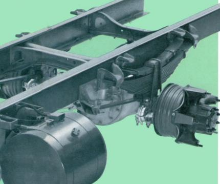
Full Vari-Rate rear springs on single axle 7500 models adjust to load conditions automatically; radius link reduces driving and braking thrusts.
