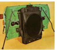
Extreme front end sheet metal, radiator, support struts and quick disconnect wiring remove as a unit for complete front-of-engine access. Entire unit allows rapid replacement of job damaged components. Helps make maintenance work easy.
