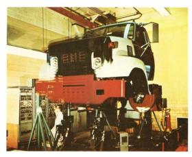
All GMC cabs are expected to take a beating in tough, everyday work situations. This split frame photo shows a test unit on the rack going through a simulated round-the-world run encountering the same type of shocks, stresses and sheet metal twisting found in the roughest operating conditions. We apply tough standards to every cab we build . . . you get the durability you expect of the Truck People from General Motors.
