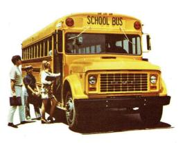
Basic School Bus Cowls adapt to most school bus bodies with a minimum of modification. Pusher type chassis are also available. A choice of automatic transmissions is available and gas or diesel power for economical operation.
