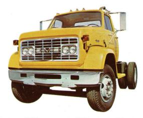
Maximum GCWs range up to 65,000 pounds. GVWs in single axle models range up to 31, pounds; in tandems, up to 48,500 pounds. Full air brakes a standard.
