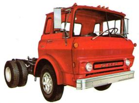
Set-back front axle design improves weight distribution and driver visibility on crowded city streets. Available with a wide range of gasoline or diesel engines for straight truck or tractor application.
