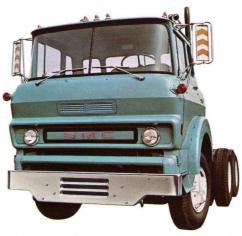
Maximum GCWs range from 40,000 to 65,000; GVWs from 27,500 to 33,000 pounds in single-axle models. GCWs in tandem axle models up to 76,800 pounds.
