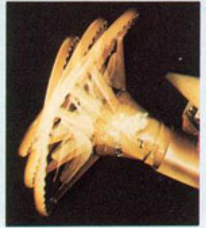
Seven-position tilt steering wheel. Adjustable so a driver can select a comfortable position; easier to enter and exit.
