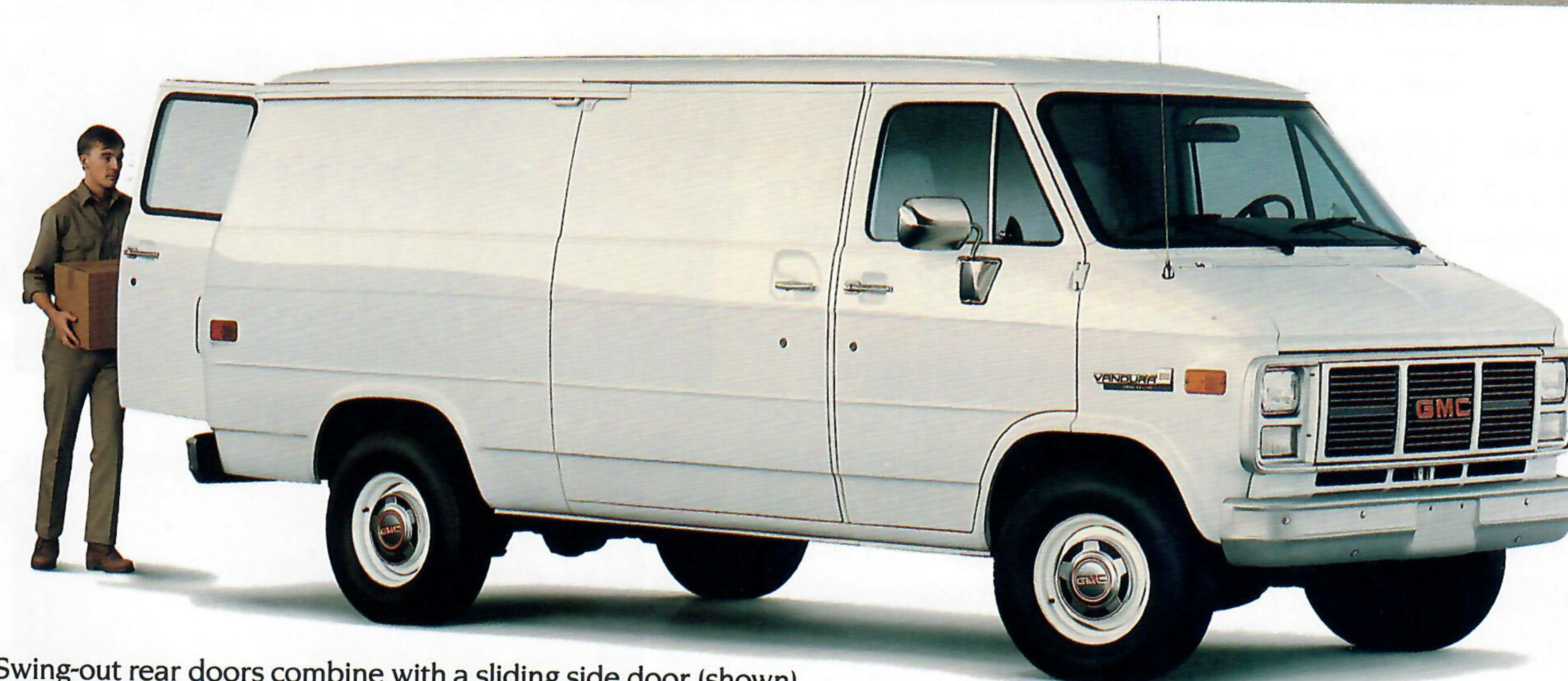
Swing-out rear doors combine with a sliding side door (shown) (or swing-out side doors) for easy loading and unloading
