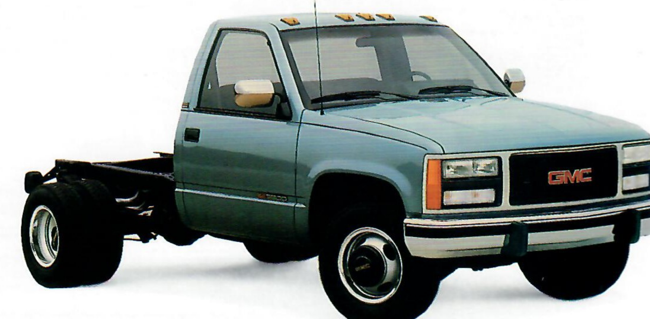
Series C-3500 131.5-inch wheelbase Sierra Regular Cab Chassis-Cab shown with new standard dual rear wheels
