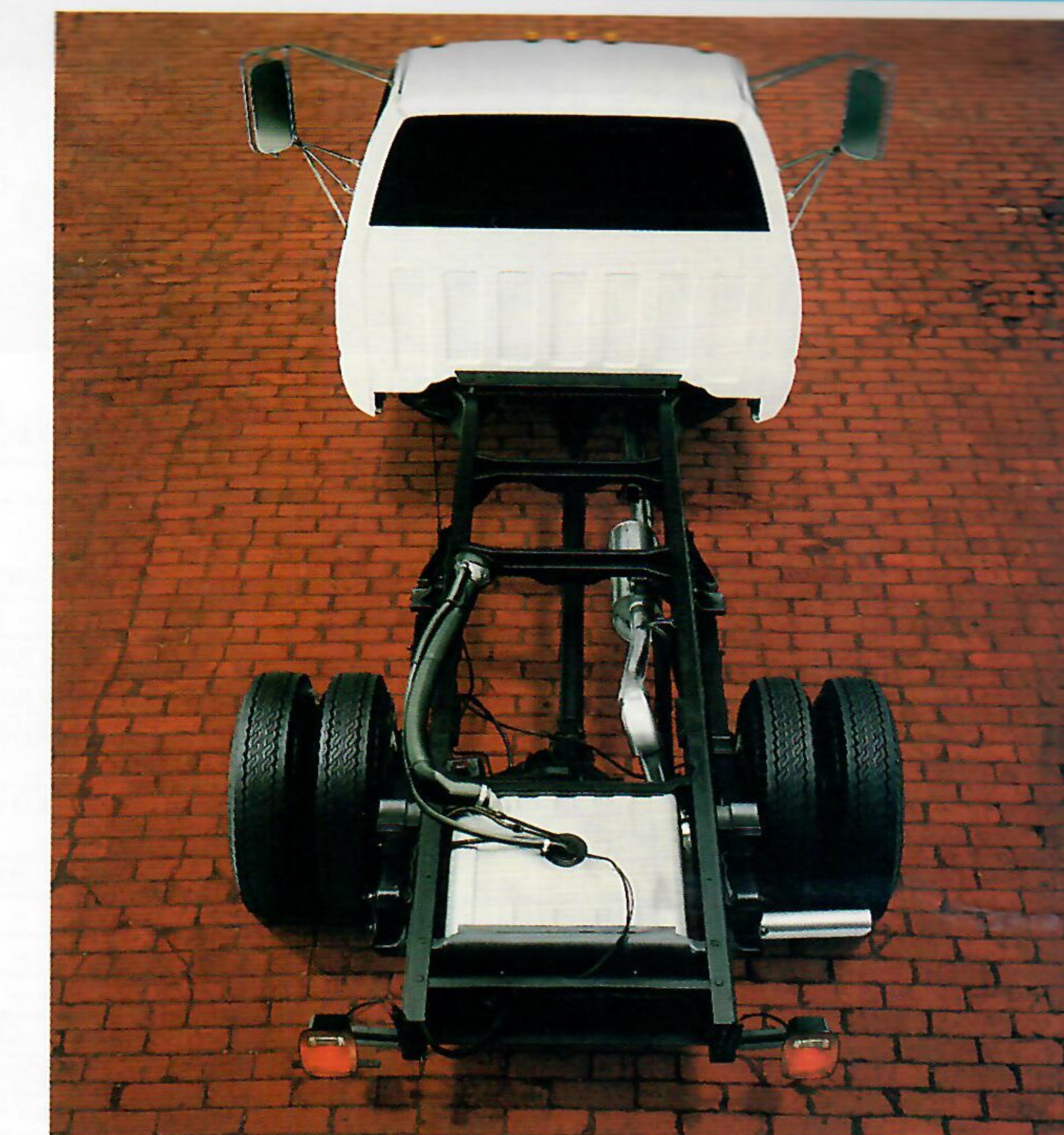
New Series 3500 HD Chassis-Cabs feature straight, flat, 34-in wide frame rails for easy mounting of commercial bodies
