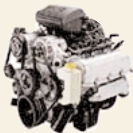
An all-new 12-valve, SOHC 3.7L Power Tech V6 is standard on Limited Edition (optional on Sport). For smooth operation, the V6 features a centrally mounted eccentric balance shaft.
