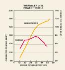
Wrangler's 2.5L Power Tech I-4 engine delivers 120 horsepower @ 5,400 rpm and 140 lb-ft of torque @ 3,500 rpm.
