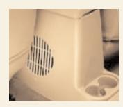
Felt but not seen; the available eight-inch subwoofer (standard on Sahara) is nicely tucked away in the full-floor center console.
