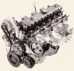
The 4.0L Power Tech I-6 has efficiency, reliability and durability thanks to a rail coil distributorless ignition system, an efficient "splitter vane" water pump, less restrictive exhaust manifold and durable multilayer steel exhaust gasket.
