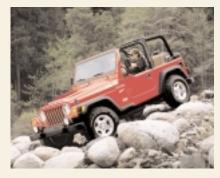
The spirit of a true rock climber resides under the skin of every Wrangler. Its stout transfer case features authentic low-range 4WD operation, axle ratios are geared low enough for rock crawling, and generous approach (44.3 degrees), breakover (25.4 degrees) and departure (32.1 degrees) angles make coming and going easy.
