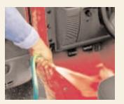
Thanks to removable carpet, water-resistant seat fabrics and drain plugs in the floor, Wrangler's interior can be hosed out after your offroad adventures.
