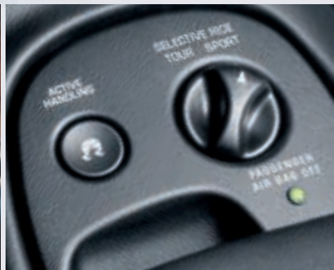
Magnetic Selective Ride Control ™ has two settings: Tour , providing a controlled, smooth ride and Sport , giving the driver a greater feel of the road surface. Optional on all coupes and convertibles. Not available on Z06.
