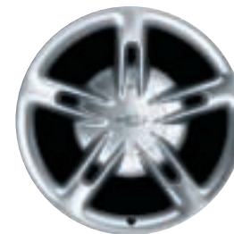
STERLING-SILVER PAINTED ALUMINUM WHEELS: 19" x 8" FRONT, 20" x 10" REAR. STANDARD ON SSR 1SA AND 1SB.
