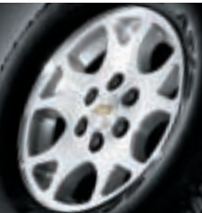
17-INCH Z71 SIX-LUG, MACHINED CAST-ALUMINUM WHEEL
