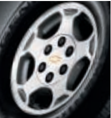
NEW 16-INCH LS AND LT HALF-TON SIX-LUG CAST-ALUMINUM WHEEL
