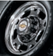
16-INCH LS AND LT THREE-QUARTER-TON EIGHT-LUG, POLISHED FORGED-ALUMINUM WHEEL WITH BRIGHT CHROME FINISH CENTER CAPS
