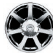
17" x 7.5" cast-aluminum, mirror polish finish. Standard on Luxury Sport Package.
