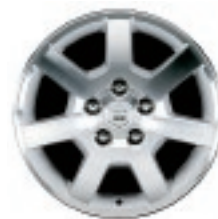
16" x 7" cast-aluminum machined-bright finish. Standard on Luxury Package.
