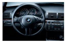
A three-spoke leather-wrapped multi-function sport steering wheel lets you keep both hands on the wheel while adjusting audio settings, cruise control and the accessory phone.
