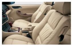
**Eight-way adjustable seats** (including 2-way headrests) firmly support the driver and front passenger over long distances. Front seat bolsters help eliminate "submarining" during sudden stops. (325Ci; 330Ci has eight-way power seats)
