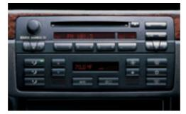
BMW anti-theft AM/FM stereo/CD/MP3 audio system produces full, rich sound through 10 speakers. Includes Radio Data System (RDS), Auto-Store; pre-wired for a BMW six-disc CD player/changer¹ and compatible with auxiliary audio input adapter¹ for audio connection of portable music players, standard. (325Ci; Harman Kardon stereo system standard in 330Ci)
