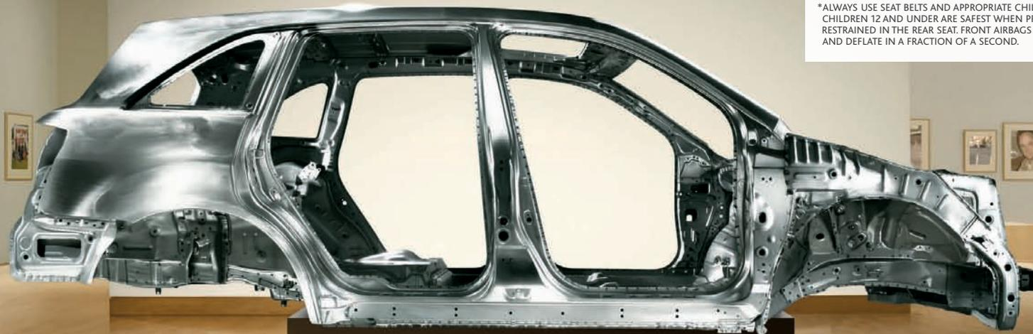
**ADVANCED COMPATIBILITY ENGINEERING™ (ACE™)** DESIGNED TO ENHANCE OCCUPANT PROTECTION AND CRASH COMPATIBILITY IN FRONTAL COLLISIONS, ACE UTILIZES A CONNECTED NETWORK OF STRUCTURAL ELEMENTS TO DISTRIBUTE CRASH ENERGY MORE EVENLY THROUGHOUT THE FRONT OF THE VEHICLE.
