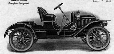
MOTOR—3½ x 4 inches. IGNITION—Dual, Magneto and Battery. TRANSMISSION—Sliding Gear, three speeds and reverse. WHEELBASE—93 inches. WHEELS—Artillery pattern. TIRES—30 x 3½ inches. SPRINGS—Half elliptic front, three-quarter elliptic scroll rear.
