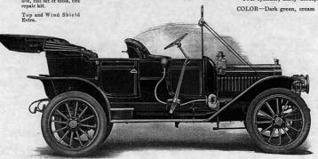
MOTOR—4¼ x 4¼ inches. IGNITION—Dual, Magneto and Battery. TRANSMISSION—Sliding Gear, three speeds and reverse. WHEELBASE—110 inches. WHEELS—Artillery pattern. RIMS—Quick Detachable. TIRES—34 x 4 inches. SPRINGS-Half elliptic front, three-quarter elliptic scroll rear.
