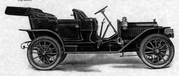
MOTOR—4½ x 4½ inches. IGNITION—Dual, Magneto and Battery. TRANSMISSION—Sliding Gear, three speeds and reverse. WHEELBASE—110 inches. WHEELS—Artillery pattern. RIMS—Quick Detachable. TIRES—34 x 4 inches. SPRINGS-Half elliptic front, three-quarter elliptic scroll rear.
