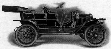
MOTOR—8½ x 4 inches. IGNITION—Dual, Magneto and Battery. TRANSMISSION—Sliding Gear, three speeds and reverse. WHEELBASE—93 inches. WHEELS—Artillery pattern. TIRES—30 x 3½ inches. SPRINGS—Half elliptic front, three-quarter elliptic scroll rear.
