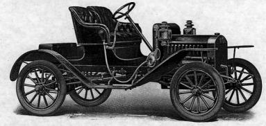
MOTOR-4½ x 4 inches. IGNITION-Dual, Magneto and Battery. TRANSMISSION-Planetary Gear. WHEELBASE-86 inches. WHEELS-Artillery pattern. TIRES-28 x 3 inches. SPRINGS-Full elliptic, front and rear.
