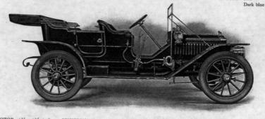
MOTOR-4½ x 4½ inches. IGNITION—Dual, Magneto and Battery. TRANSMISSION—Sliding Gear, three speeds and reverse. WHEELBASE—110 inches. WHEELS—Artillery pattern. RIMS—Quick Detachable. TIRES—34 x 4 inches. SPRINGS-Half elliptic front, three-quarter elliptic scroll rear.
