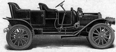
MOTOR—4 x 4 inches. IGNITION—Dual, Magneto and Battery. TRANSMISSION—Sliding Gear, three speeds and reverse. WHEELBASE—104 inches. WHEELS—Artillery pattern. RIMS—Quick Detachable. TIRES—32 x 3½ inches. SPRINGS—Semi-elliptic front, three-quarter elliptic secoil rear.
