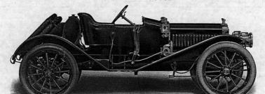
MOTOR—4½ x 4½ inches. IGNITION—Dual, Magneto and Battery. TRANSMISSION—Sliding Gear, three speeds and reverse. WHEELSASE—110 inches. WHEELS—Artillery pattern. RIMS—Demountable. TIRES—34 x 4 inches. SPRINGS-Half elliptic front, three-quarter elliptic scroll rear.
