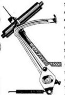
The clutch is operated by the pedal acting through a stamped lever which is adjustable in relation to the pedal position. Pedal motion is transmitted to the clutch fork through this lever. The pecals are mounted on a shaft which is provided with flats at its end. It bears in a two bolt bracket which, with the bolt through the shaft, forms a more rigid mounting which lends itself to economical production.
