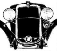
plated. A black enameled, beaded panel at the bottom surrounds the starting orank hole. The new radiator design appears to be much higher and the sides appear to have more curvature. The upper panel is somewhat narrower and has greater curvature at the rear edge. The
