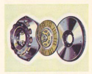
CLUTCH—Durable, dependable, chatter-free clutch operation is assured in the Kaiser by extra-large clutch facing area, sealed ball release bearing design, Easier operation... more miles of silky-smooth performance.
