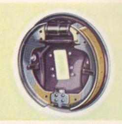
BRAKES—Self-centering, full-floating hydraulic brakes use an advanced braking principle proved in war-time combat vehicles. Soft, gliding stops in traffic, and instant toe-tip control in sudden, severe applications.
