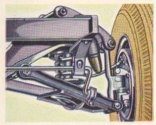
SPRINGING—Kaiser independent-suspension front coil springs are longer this year, easier-acting. Large, vertically-mounted, direct-acting shock absorbers inside the springs further contribute to "the ride you'll never forget." You glide over bumps you can see but can't feel.
