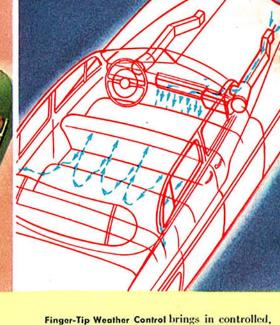
draftless fresh air. Used with the new Mercury heater (optional\*), it lets you select the exact amount of heat and fresh air you want. Prevents window fogging, too.
