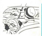
A fog-free windshield—As only fresh, relatively low-humidity, outside air is used when heating, and as stale air is rapidly removed before moisture has a chance to condense, the windows rarely fog or steam up, even in winter.
